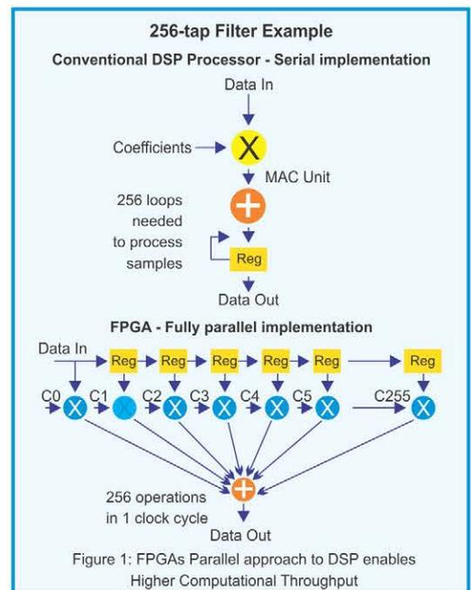
Figure 1: FPGAs Parallel approach to DSP enables Higher Computational Throughput
